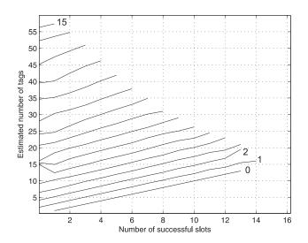
Fig. 6. Linear model behavior of the frame (L = 16) obtained experimentally in [21]. Lines represent collisions, 0-15, down-up.  $16^{th}$  line is a point, because all-collision scenario results with 0 successful slots
