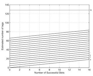
Fig. 7. Linear model behavior of the frame (L = 16) obtained from combinatorial model. Lines represent collisions, 0-15, down-up. Last line, for all collision scenario is in this case  $n = 2^{Q_{current frame}+3} = 2^7 = 128$
