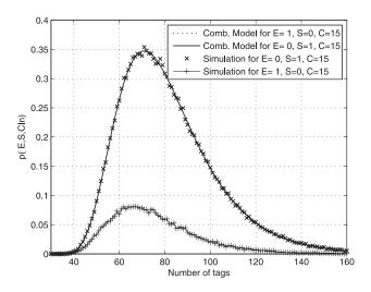
Fig. 5. Results of FSA simulation and Combinatorial model in (14). The maximum of depicted distributions  $p(E, S, C \mid n)$  is used as estimation of number of tags within interrogation area.
