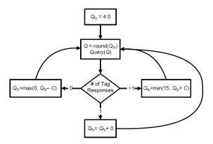
Fig. 3. Q-Selection Algorithm sequence diagram from UHF-GEN2-RFID [6]
